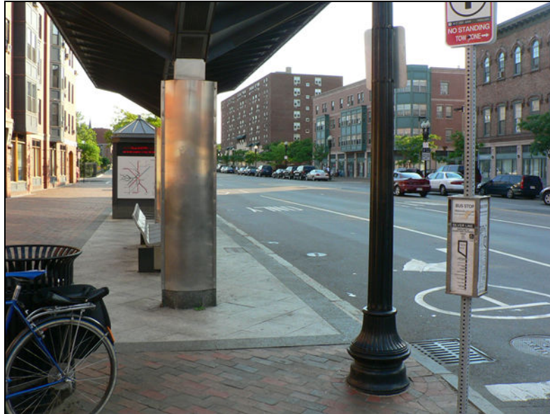
Figure 8: Massachusetts Avenue Inbound Stop in 2005 (Note: wider sidewalk, specialty pavers, historic light pole, bench, shelter, information box on sign post, kiosk with route map, and combined bus and right turn lane)
